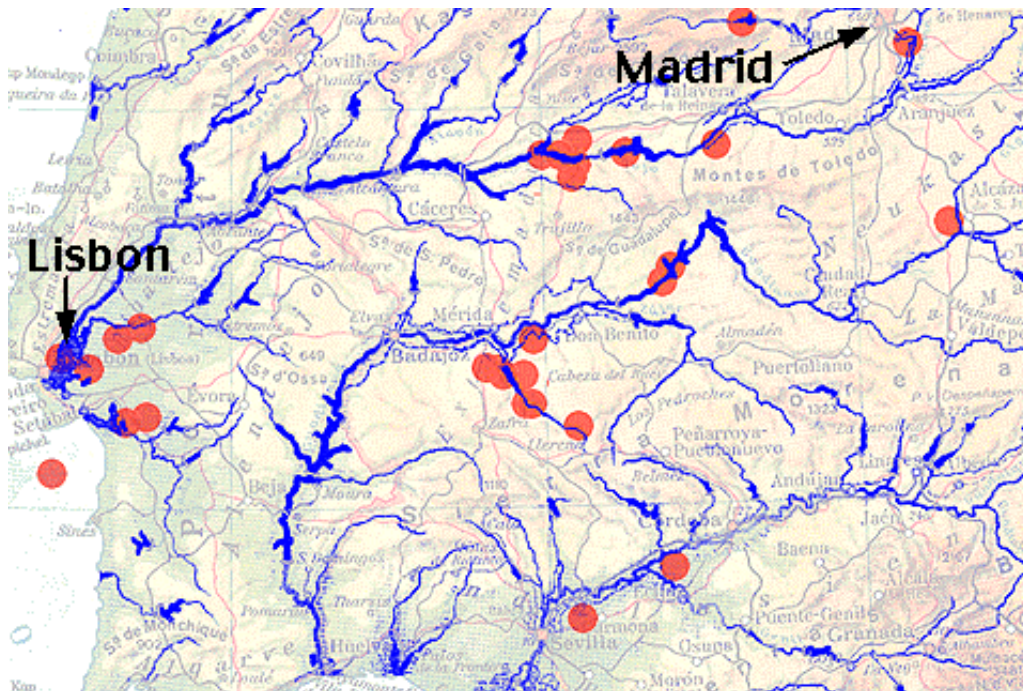
Fig. 1.1. In the May 20, 2003 dx opening, sixty percent of the radio paths between the Canary Isles and central Europe show midpoints which appear to correlate to the position of lakes and major rivers in Spain and Portugal [1].
