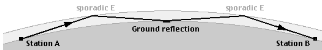
Fig. 1. Schematic view of a double hop sporadic E QSO.
