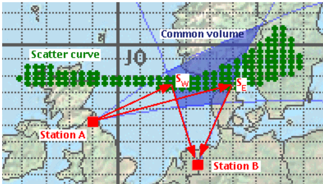
Figure 11. Auroras extending in a large geographical area (green) may cause backscattering from various regions within the common scatter volume (blue).
